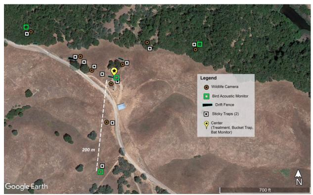
**Figure 3.** Diagram from one treatment site (HREC1) demonstrating the distribution of monitoring equipment. Each site consists of three transects extending out to 200 m, with the spacing of monitors based on taxonomic and equipment considerations (see text). One transect (in this case, the NW transect in the upper left) contains a higher density of monitoring equipment closer to the treatment source to test for finer scale and distance threshold effects.
